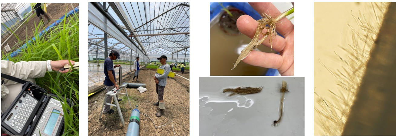
Figure 1. Examples of some of the methods. From left to right, stomatal conductance using a porometer (AP4), leaf water potential using a Scholander pressure chamber (Soil Moisture), root preparation for root hairs analysis, example root hair picture.
