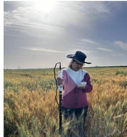
Installing soil tubes and taking soil moisture data by using the FDR soil moisture sensor
