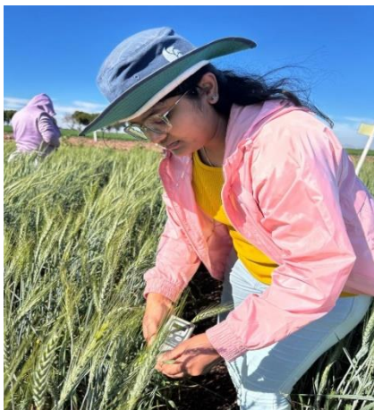
PRI and leaf greenness data were measured by using plant pen PRI and SPAD meters, respectively
