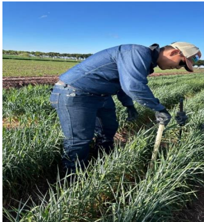
Installing soil tubes and taking soil moisture data by using the FDR soil moisture sensor
