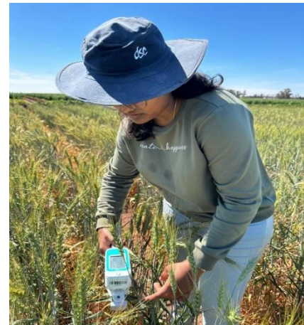
Photosynthetically Active Radiation (PAR) and Stomatal Conductance data were collected by using Ceptometer and Porometer, respectively
