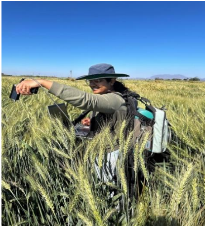
Spectral Reflectance Indices were collected at both the canopy and leaf levels using the ASD machine
