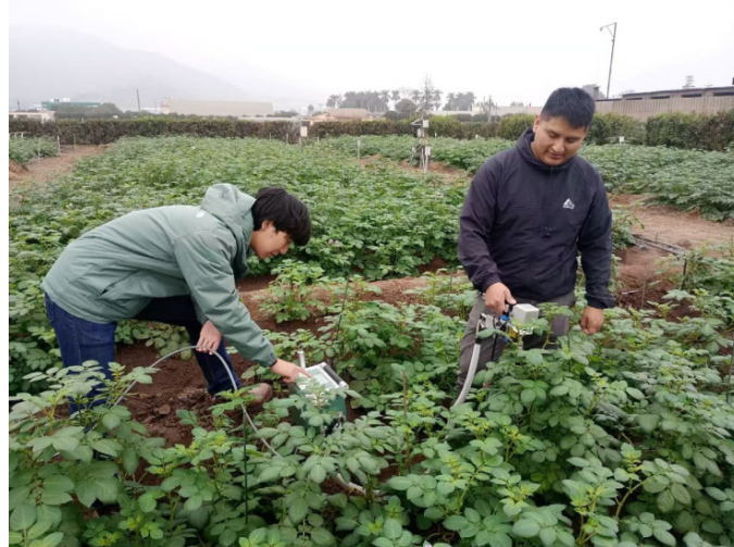
Figure 1. Me and Johan using the LI-COR 6800 system to measure crop photosynthesis
