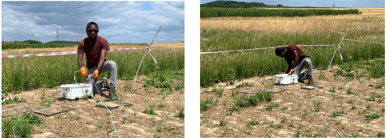
Figure 2: Connecting tubes to static chambers at Oberer-Hardthof
