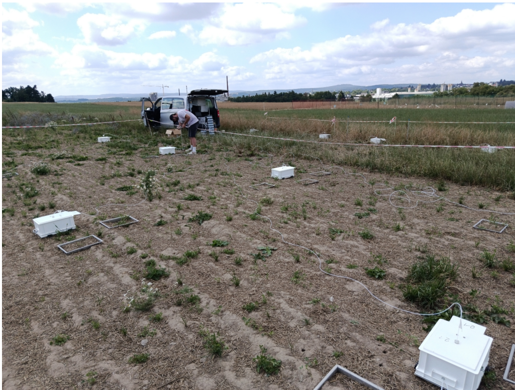
Figure 1: Greenhouse gas measurements using static chamber approach, from land previously occupied by a chicken mobile barn at Oberer-Hardthof
