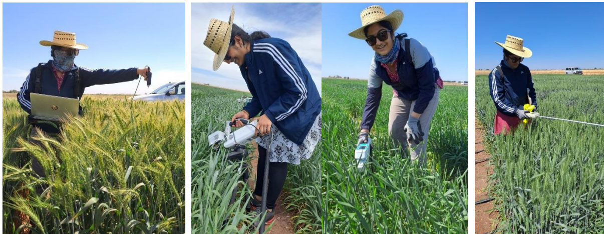
Fig.3 Canopy reflectance measured with ASD Field Spec® 3 (left), photosynthetic traits assessed using LICOR-6800 and Porometer/Fluorometer (middle) and light interception measured with AccuPAR LP-80 (right).
