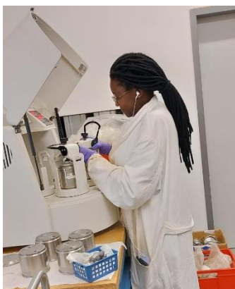
Setting up samples for ball milling
